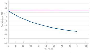
MDF-25V268E Pull Down Test at Ambient
