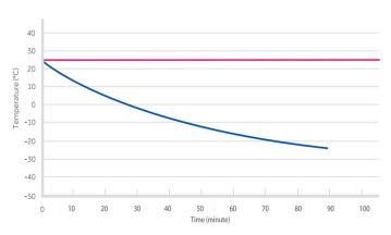
MDF-25V268E Pull Down Test at Ambient
